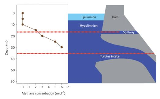
Diagram of the Tucuruí Dam, with methane (CH4) in the water indicated in the graph at the left. Water passing through the spillways and turbines is taken from depths with high methane concentrations. This methane is released into the air below the dam. Source: Fearnside & Pueyo (2012).
