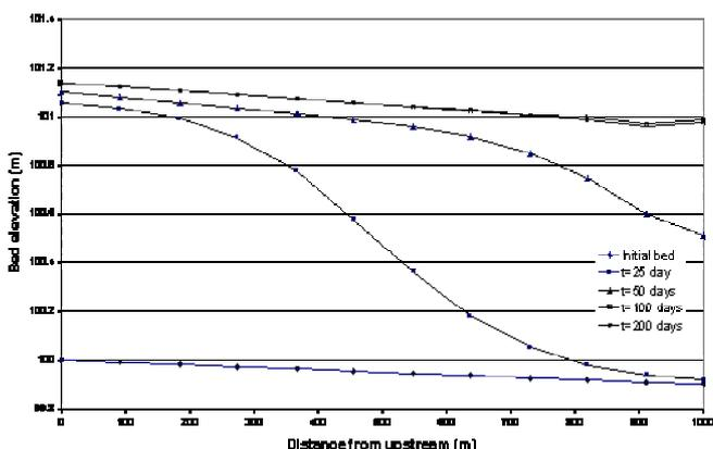
Figure 4. Initial bed and computed channel bed profiles at different times
