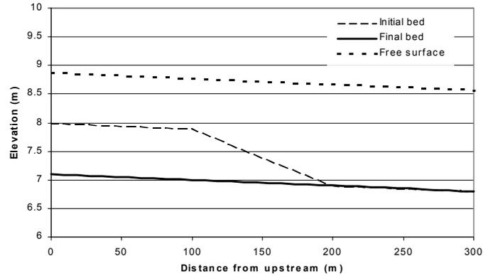
Figure 2. Initial bed, computed equilibrium bed and water surface
