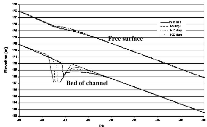
Figure 17. Miribel channel: initial bed, computed equilibrium bed and water surface.
