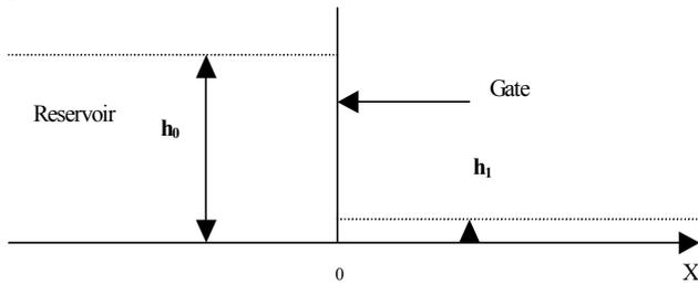
Figure 7. Idealized dam-break problem,  $h_0$  and  $h_1$  are the initial depths upstream and downstream of the dam before failure.
