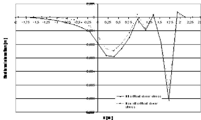
Figure 12. Bottom level evolution with nil or non nil critical shear stress:  $\Delta x = 20$  cm,  $D_{char} = 1$  m,  $CFL = 0.5$ ,  $t = 2$  s
