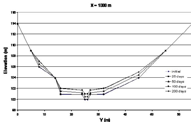
Figure 5. cross-section deformation: a)  $x = 0 \text{ m}$ , b)  $x = 1000 \text{ m}$
