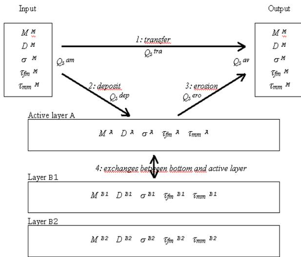
Figure 1. Representation of the sharing of sediments inside one cell (Balayn 2001)
