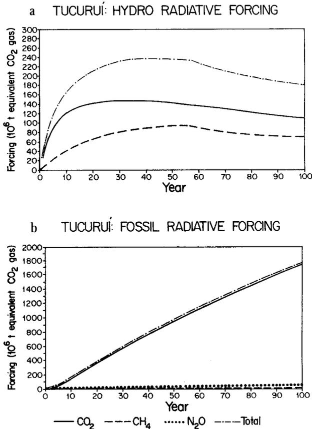
**Figure 5** Tucuruí: radiative forcing of the atmospheric loads of greenhouse gases (a) from the hydroelectric project, (b) from fossil fuel displaced by Tucuruí. The centre of gravity of the total radiative forcing curve is at year 52 for hydroelectric emissions and at year 67 for fossil-fuel emissions, a difference of 15 years.
