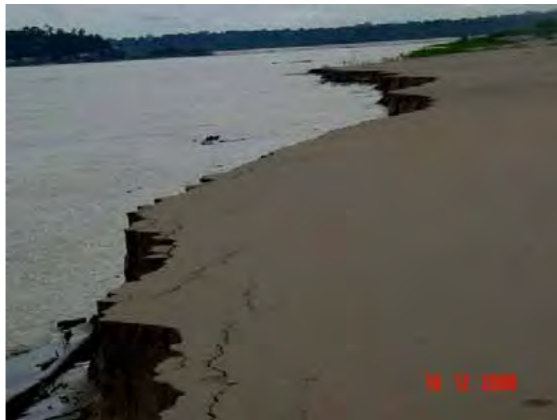
Figure 4 - Sand bar downstream of Teotonio Rapids composed of clean sand no trace of silt or clay is eroding with increasing river discharge of 12,000 m 3 /s on December 12, 2007.
